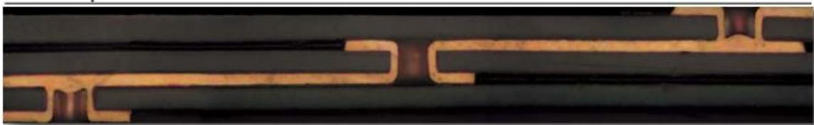
· 100 micron laser drilled microvias
