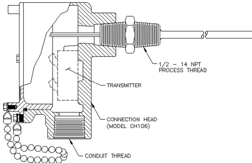
2. Slide the probe, tip first, into position and thread the fitting into the process connection. Tighten using a 7/8" open-end or adjustable wrench.
