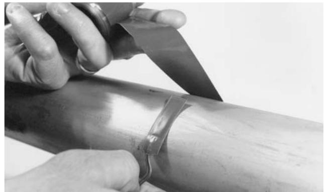
When properly insulated, Thermal-Ribbon time response and accuracy are equal to immersed thermometers
