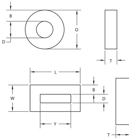
**Coil shape:** Coils may have round, rectangular, oval or irregular shapes. Coils with reverse radius of curvature (banana shaped) must be formed after winding, so their B dimension must be thin enough to be bent without straining wires. Shown below are typical wound coils before lamination.
