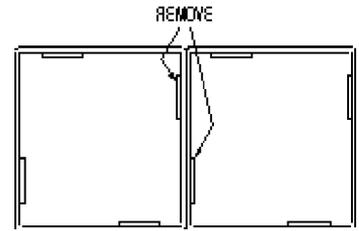
Prepare the panel by cutting and deburring the required opening.
