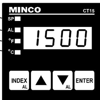
Decimal point flashes while ramping function is active.
