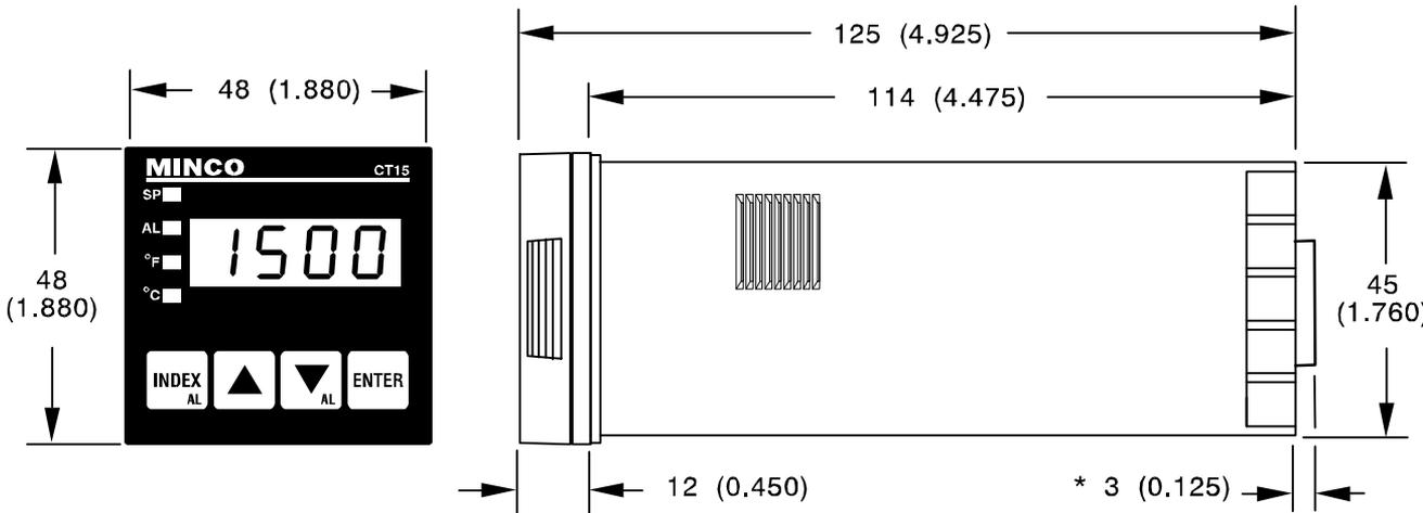
Panel cutout for all models 45 mm X 45 mm (1.775" X 1.775"). Allow for 13 mm (0.5") clearance at the rear of instrument.
