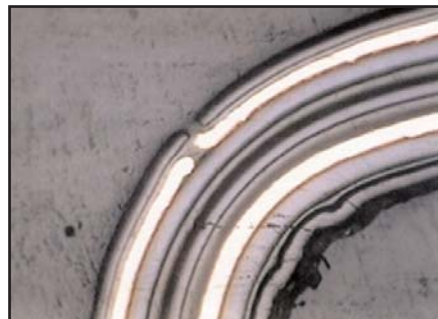
Figure 2: If a circuit is not properly designed and handled, outer layers can tear or crack and inner layers can wrinkle or delaminate
