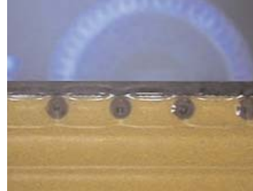
Figure 11: Stitched vias, like through holes, should be kept out of bend area
