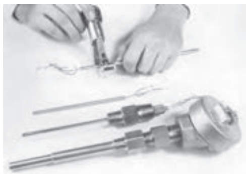
Shorten probes easily with a tubing cutter
