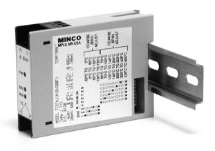
The Model TT274 is a 2-wire temperature transmitter for types J and K thermocouples. The transmitter converts the thermocouple's millivolt signal to a 4 to 20 mA DC current signal. Because this current signal is immune to leadwire and electrical noise, the TT274 lets you obtain accurate temperature readings from thermocouples thousands of feet away. An ordinary twisted pair of wires carries both the temperature signal and power for the transmitter's electronics.
