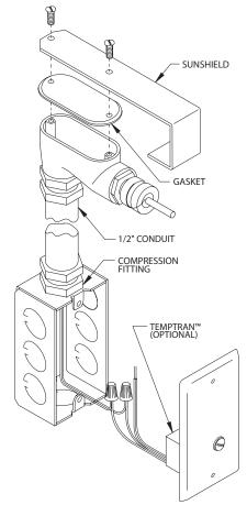
Figure 3: Outside air thermometer
