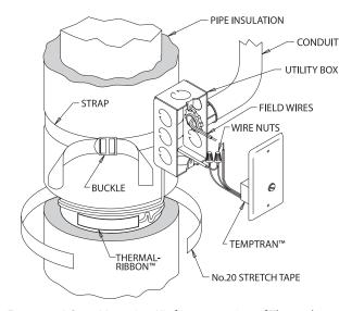
Figure 11: AC766 Mounting Kit for connection of Thermal-Ribbon thermometer and Temptrans, mounted on pipe
