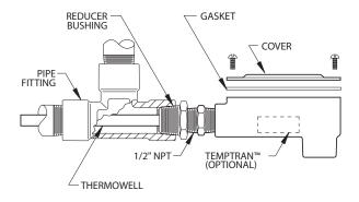
Figure 9: Fluid immersion thermometer in a small pipe
