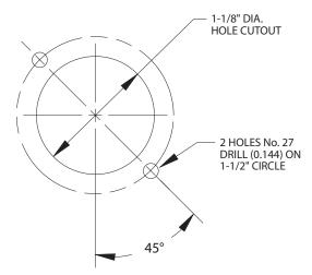
Template 3: Duct air thermometer
