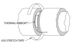
Figure 10: Thermal-Ribbon thermometer mounted on pipe
