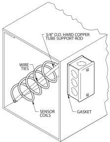
Figure 6: Bendable averaging thermometer, Installation A
