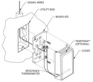
Figure 1: Room air thermometer with Temptran
