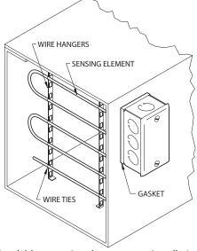
Figure 7: Bendable averaging thermometer, Installation B
