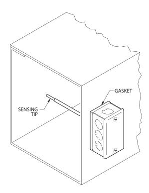
Figure 4: Duct air thermometer
