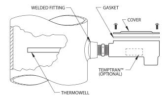
Figure 8: Fluid immersion thermometer in a large pipe
