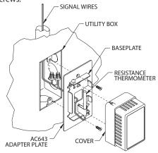
Figure 2: Compact room air thermometer
