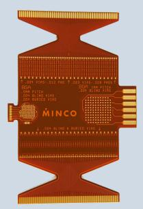
Under vibration and/or high acceleration, a flex circuit's ductility and low mass will reduce the impact upon itself and solder joints. By contrast, a PCB's higher vibrational mass will increase stresses upon itself, components and solder joints.
