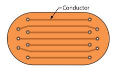
**Conductor spacing**: The distance between conductor strands or pads. A certain minimum conductor spacing must exist in order to prevent conductors from shorting together.
