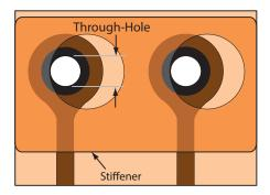
or cover access hole is flush with the edge of a through-hole.
