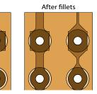
between conductors and pads are to be avoided by using fillets to minimize the concentration of stress at the interface.
