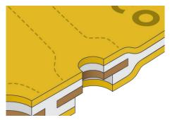
**Nesting**: Designing circuits so that they lay closely together on a panel during production. This maximizes the usage of panel space, which minimizes production cost.
