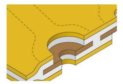
**Minor access hole**: An access hole (see "Access hole") that exposes only a very small portion of a conductor pad, used on holes where a solder pad is not needed or desired. The cover hole must still be larger than the through-hole to allow for normal registration tolerances. Generally against a component or a stiffener.
