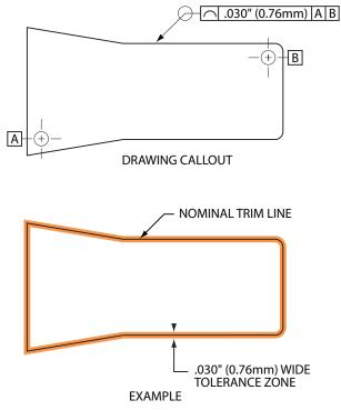
profile tolerance zone. The circuit trim line could vary anywhere inside the zone.
