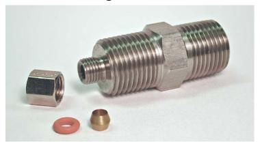
An O-ring and/or a compression ring are supplied with each fluid seal fitting. Either the O-ring or the compression ring may be installed as the seal. The O-ring is silicone rubber and is resistant to petroleum oils, and most hydraulic fluids. The compression ring is recommended where there is longitudal vibration or force on the probe.
