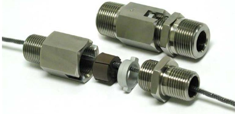
Minco's multi-conductor feedthroughs are designed for use in applications which require several conductors, probe type sensors or cables to pass through a housing or bulkhead within a small area. Their construction allows the fittings to be used in pressure applications up to 50 PSIG.
