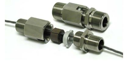
Minco's multi-conductor feedthroughs are designed for use in applications which require several conductors, probe type sensors or cables to pass through a housing or bulkhead within a small area. Their construction allows the fittings to be used in pressure applications up to 50 PSIG.
