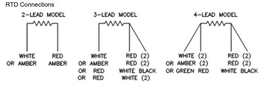
The above color code is Minco's standard colors, but alternatives can be used. Refer to the model specification drawing for the actual color code.
