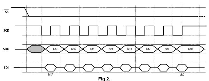
Note: Slave Select (SS) should be low for the entire transmission of 9 bytes (packets).
