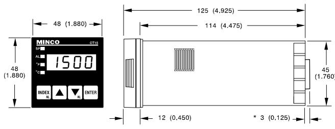
Panel cutout for all models 45 mm X 45 mm (1.775" X 1.775"). Allow for 13 mm (0.5") clearance at the rear of instrument. \*Present for SSR and 5 VDC output.
