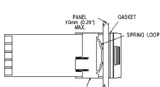
MOUNTING COLLAR (SHOWN IN POSITION) SLIDE COLLAR ONTO THE HOUSING BEFORE WIRING THE REAR TERMINALS
