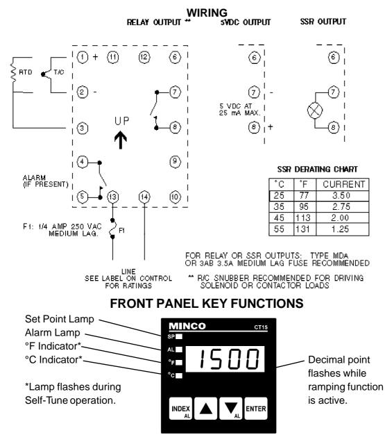
The 1500 Series controls have one display. The display must occasionally switch to show a complete message or menu item and its value. The normal display shows just the temperature and does not switch. While showing a menu item, the display will alternate between the menu item and the item value. If the UP arrow, DOWN arrow, or ENTER keys are pressed, the display immediately switches to display the item value.
