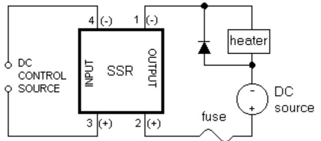
Figure 2 Wiring Diagram
