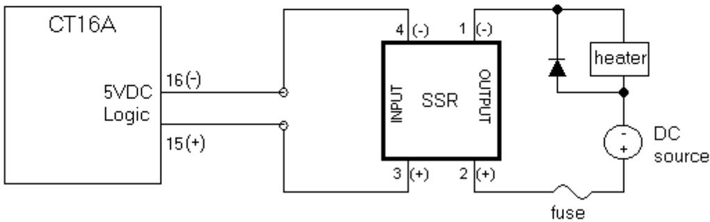
CT16A has two outputs. Output A is shown in the diagram. Output B is wired in a similar manner, but uses pins 18(-) and 17(+).
