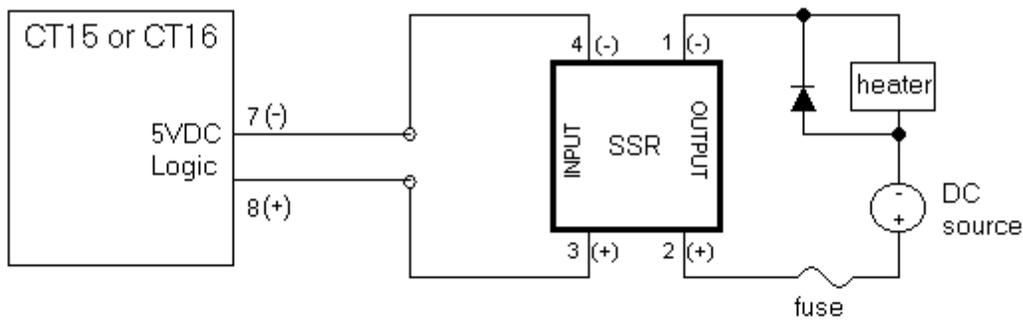
CT16 has the option for a second logic output. The optional output will be wired in a similar manner, but uses pins 9(-) and 10(+).
